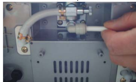
1/4" White Hose to Tap Water Inlet Port
