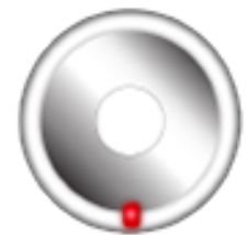
0% Capacity + Alarm Replace Immediately! Red
